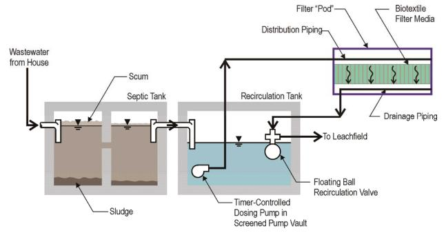
Figure 6-4 – Biotextile Filter Schematic
