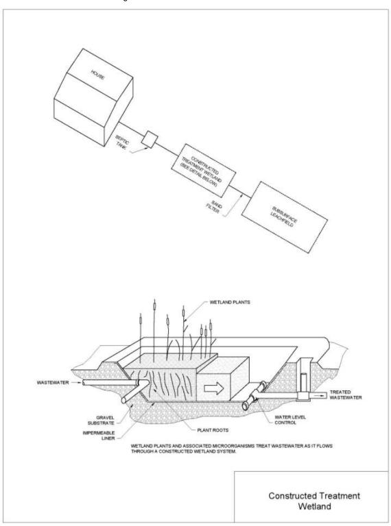
Figure 6-6 – Constructed Treatment Wetland
